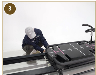
3 Connect frame half with cross member
