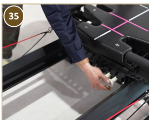
35 Secure adjustment knob at carriage stopper
