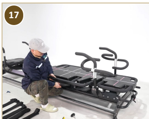
Check longitudinal alignment of both carriages
