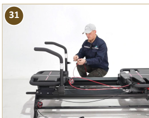
31 Pulley final assembly on the carriage frame
