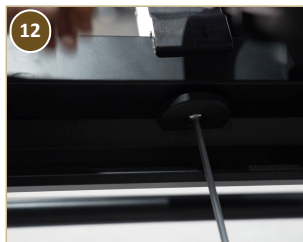
Tighten screw at the support frame
