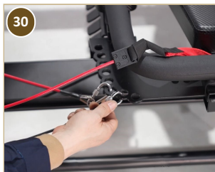
30 Run iron rope over the pulley wheel
