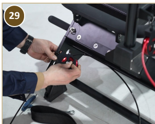
29 Screw pulley to the frame
